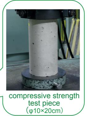
compressive strength test piece (φ10×20cm)
