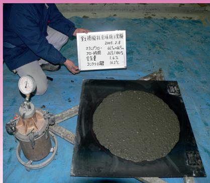
Slump flow test
