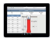
The point of the tremie pipe and the concrete height are visualized.
