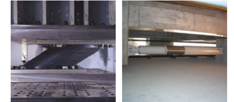
Laminated rubber bearing
